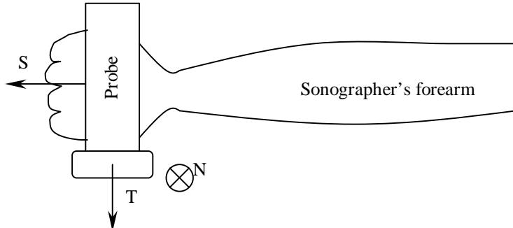
**Figure 1.** The sonographer as he holds the probe, defining natural axes for the representation of the scene.
