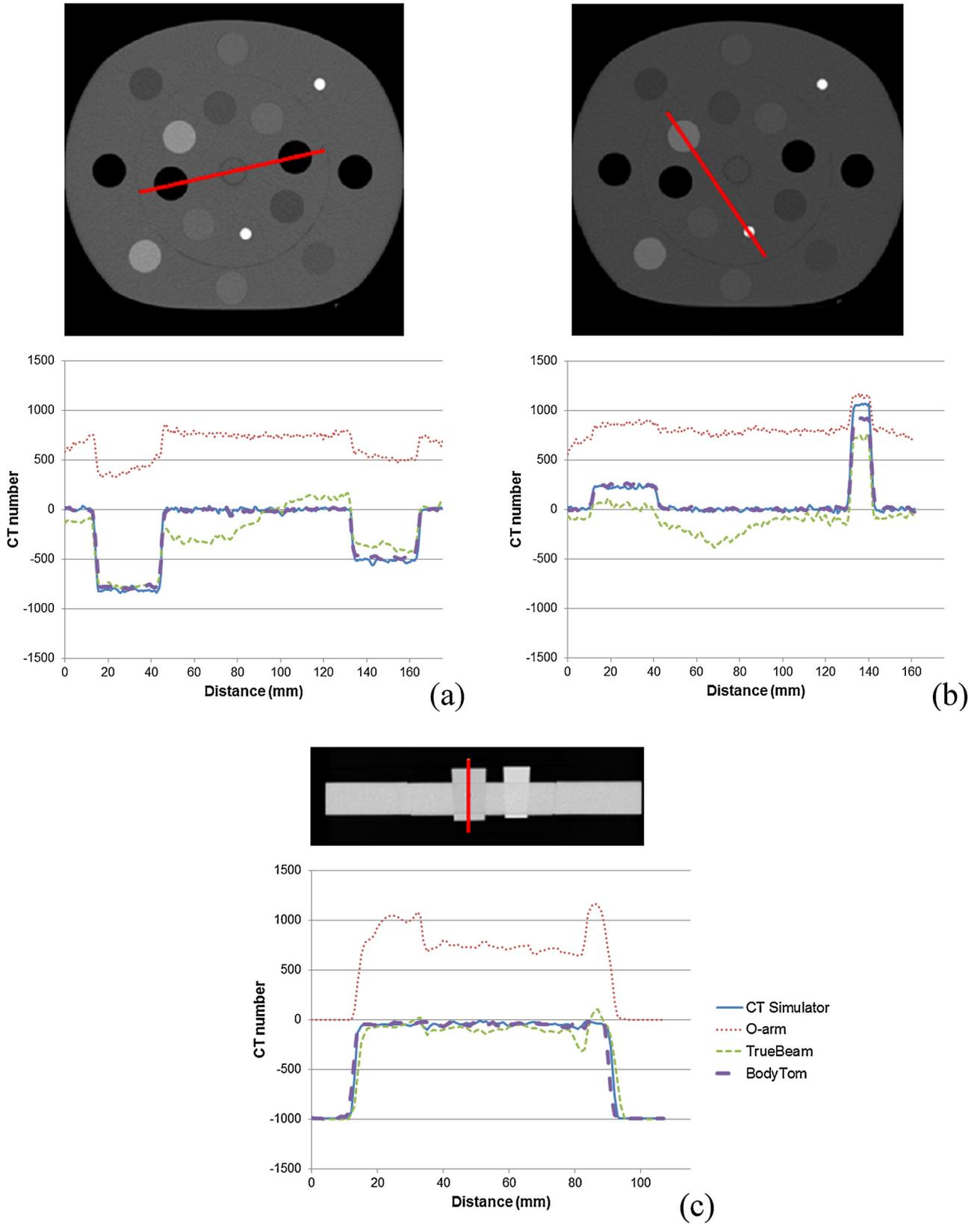
Fig. 5. Electron density phantom profiles for each CT scanner: (a) Lung inhale – Plastic Water – Lung exhale, (b) Trabecular bone 200 mg/cc – Plastic Water – Dense bone 800 mg/cc, (c) Air – Breast 50% gland/50% adipose – Air. Values shown for O-arm profiles are not corrected.
