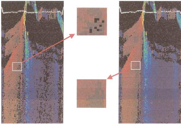
Fig. 1. Image enhancement obtained with the selective median filter (kernel size  $11 \times 11$ ). Left = original image, right = filtered image. Zoomed regions are shown to better see the difference.
