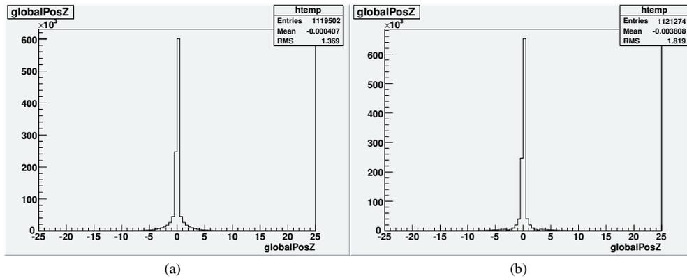
**Figure 8.** Histograms of the  $z$  position detected after one million normally incident emissions from a point source positioned at  $(0, 0, 0)$ : histogram for a continuous detector of thickness  $H = 10$  mm (a), and histogram for a pixelated detector of thickness  $H = 5$  mm (b).
