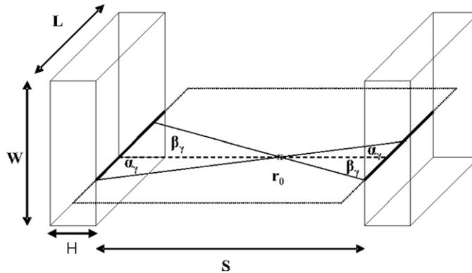
**Figure 2.** Geometrical characterization of the range of detectable emissions from the point  $\mathbf{r}_0$  within the plane  $xy$ . The angles  $\alpha_\gamma(\mathbf{r}_0)$  and  $\beta_\gamma(\mathbf{r}_0)$  define the maximum and minimum  $\gamma$  detectable LORs within the plane  $xy$ .
