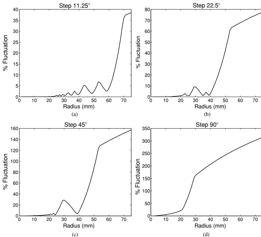
**Figure 7.** Fluctuation of the normalizing term (computed as the ratio of the peak-to-peak difference to the mean value) along a circumference as a function of its radius for the different rotation configurations (rotation angular steps of 11.2 (c), 22.5 (d), 45 (e) and 90° (f) of the YAP-PET scanner. The variation is negligible for the smallest rotation steps but can reach values of more than 300% for the 90° rotation case.
