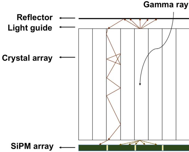
Fig. 1. Schematic representation of the DOI encoding method.
