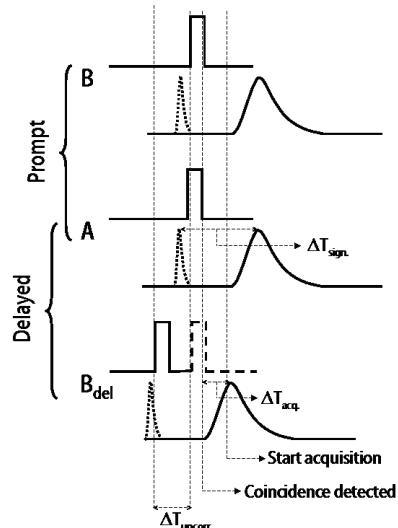
Fig. 1. Timing scheme for the standard acquisition of the Anger signals in a prompt and in a delayed (A vs. B<sub>del</sub>) coincidence (opposing detectors A and B are considered). To be able to acquire B side signals in a delayed coincidence  $\Delta T_{\text{sign.}}$  should be larger than  $\Delta T_{\text{uncorr.}} + \Delta T_{\text{acq.}}$ .
