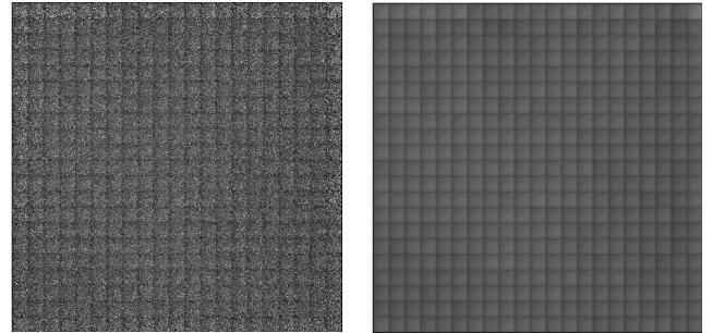
Fig. 6. Comparison of the delayed coincidence planograms obtained as directly measured (left) and by applying equation (2) (right). Planograms are not normalized for LOR efficiency.
