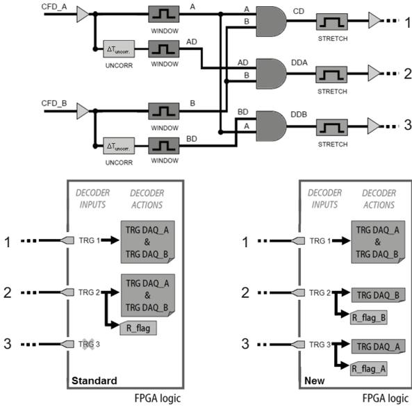
Fig. 3. Implementation of the new delayed window approach in a 1 vs. 1 modules dual head system. In this case the coincidence network scheme is fixed (top). The outputs of the coincidence network are connected to the inputs of the FPGA as numbered. The switching between the standard (bottom left) and the new (bottom right) delayed window approach is coded in the FPGA logic.
