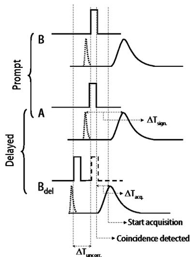
Fig. 1. Timing scheme for the standard acquisition of the Anger signals in a prompt and in a delayed (A vs. B<sub>del</sub>) coincidence (opposing detectors A and B are considered). To be able to acquire B side signals in a delayed coincidence  $\Delta T_{sign}$  should be larger than  $\Delta T_{uncorr} + \Delta T_{acq}$ .
