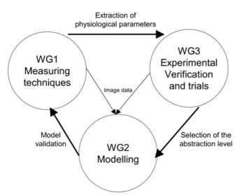
This demonstrates diagram that verification and trials not only the are end" "front of COST B21 but that an important feedback exists from verification to modelling and from modelling to method design.
